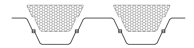
Filcor Sheet Pile Infills can be fabricated to suit all types and sizes of sheet piling
