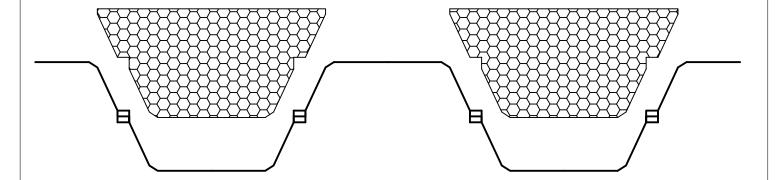
**Filcor EPS** pile infills can be fabricated to all types and sizes of sheet piling
