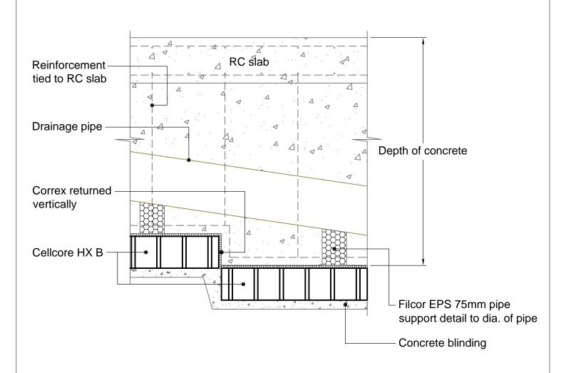
NB:- The grade of Cellcore HX B panel required may vary along the length of the drainage run as the depth of the concrete infill increases to accommodate the fall of the pipe. Detail to be read in conjunction with Standard Detail Drg No. ENG/GH/CELL/001.
