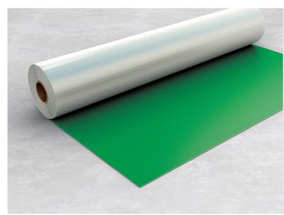
The Cordek Tri-Gas Membrane is a high performance gas membrane for use in situations where resistance to methane, carbon dioxide and/or radon gas(es) is required. It is generally used within construction applications, predominantly within the foundation design. The multilayer 0.4mm thick membrane includes an ultralow permeability aluminium foil core encapsulated between a number of additional LDPE layers and a reinforcing grid to form a single sheet membrane.
