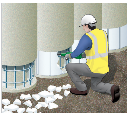
Excavated to basement level, Pilecor is removed and pile reinforcement exposed.
