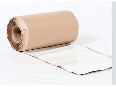
The Cordek Gas Resistant Detailing Strip is used for detailing work, when sealing a sheet membrane to penetrations e.g. steel columns, manholes, piles etc. It is manufactured using aluminium /polythene laminate coated on one surface, with an additional layer of self-adhesive polymer modified bitumen.
