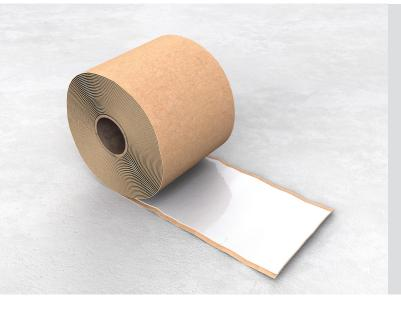
The Cordek Gas Membrane Lap Tape is typically used for the jointing of construction membranes including damp proof, radon and gas resistant sheet membranes for combined ground gas and damp proofing applications. It is manufactured using an aluminium/ polythene laminate coated on one surface with an additional layer of self-adhesive polymer modified bitumen.
