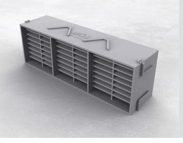
The Cordek Air Brick is designed to provide a practical method of venting ground gases from beneath a building, through the perimeter cavity wall construction with the additional use of an adjustable cavity vent. The air bricks can be connected to one of the Cordek venting systems, which when used in conjunction with a suitable membrane, provides an efficient and economical gas protection solution.
