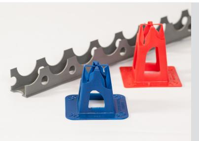
The Cordek reinforcement spacer range is designed to support reinforcing steel or mesh prior to the pouring of concrete to form a reinforced concrete structure. The spacers are left in place during the pouring of the concrete and become a permanent part of the structure upon completion.
